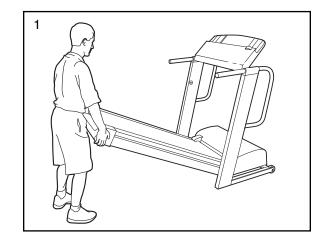
Move your right hand to the position shown and hold the treadmill firmly. Hold the lock knob with your left hand and pull it to the side. Raise the treadmill until the lock knob is aligned with the catch. Slowly release the lock knob. Make sure that the pin on the lock knob is inside of the catch.
